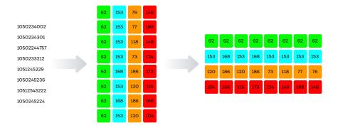
Since most instrument, or stock trade, data varies over a limited range, the area containing the most significant bits will be very compressible, holding a small range of values that repeat often. Even if the areas storing the third and low-order bytes only compress a little, the net result is a significant increase in overall compression.
