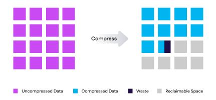
Instead of managing data in fixed-size blocks, the VAST Element Store uses byte-oriented metadata to manage blocks of any size without having to align Element Store allocation blocks with drive logical block addressing (LBA) boundaries. If a 32KB write shrinks to 14501 bytes, the VAST Element Store writes 14501 bytes to flash, and the next block starts at byte 14502. The result is that compressed data is stored waste-free, providing more usable storage capacity.
